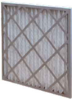
PANEL FILTERS Filter medium: Synthetic Frame: Cardboard, plastic, or metal Filter class: ISO Coarse
