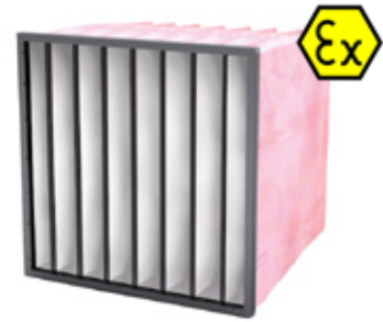
ATEX BAG FILTERS Filter medium: Multi-layered synthetic Frame: Metal Filter classe: ISO ePM2,5-65%
