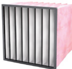
GLASS FIBER-SYNTHETIC BAG FILTERS Filter medium: Glass fiber-synthetic Frame: Metal, plastic, or wood Filter class: ISO ePM1
