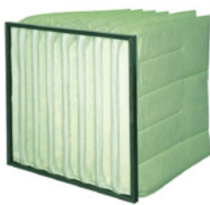
ANTIBACTERIAL BAG FILTERS Filtermedium: Meltblown polypropylene Frame: Metal or plastic Filter classe: ISO Coarse - ISO ePM1
