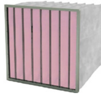
BAG FILTERS WITH CARBON Filter medium: Glass fiber Frame: Metal or wood Filter class: ISO ePM1-60%
