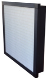
COMPACT FILTERS DCP WITH FLANGE Filter medium: Minipleated fiberglass paper Frame: Plastic Filter class: ISO EPM10-65% - ISO EPM1-80%
